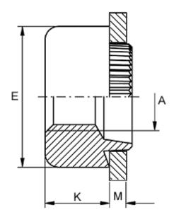
Female thread A = M14Height K = 10.0Outer diameter E = 25.0Plate thickness = 1.1 to 1.3
